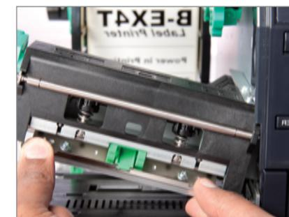
“卡扣式”打印头使装卸耗时降至最低
